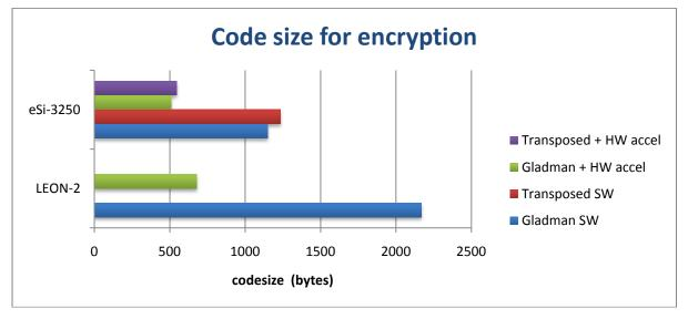
The application code is documented in this paper for reference. A 2.56x cycle count speed up is achieved for a small addition of hardware, and the encryption becomes comparable to using T-tables.
